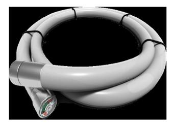
Automatic fire suppression system is a simple and cost effective fire protection of small enclosures. The system consists of a heat sensitive tube made of special plastic which is closed by a stainless steel fitting on each end. The tube has both storage and detection function which means that the extinguishing agent is stored directly in the tube and no additional storage device like cylinder is needed.
